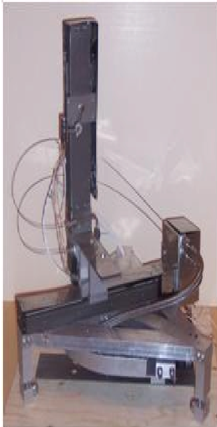
Figure A.1: Mechanical design of the system. Three stepper motors are used to position a Faraday probe in a three dimensional space.
